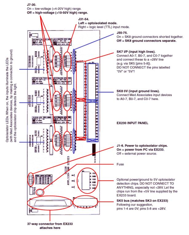
Here's an annotated circuit diagram of a single input:
