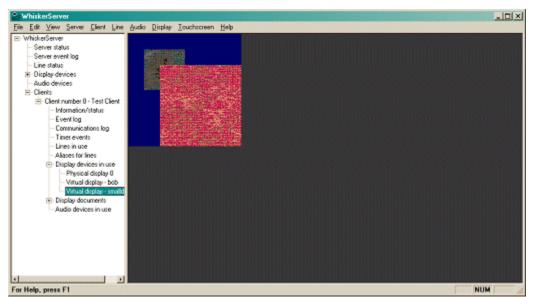
In this case, a virtual display is smaller than the server console window and scaling is off. The grey area at the edge is the area beyond that of the virtual display. Were 'Scale server's copy...' to be switched on, the picture would be enlarged to fit the server's window.
