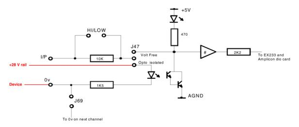
It certainly seems to work much of the time. Yet we do seem to have a high failure rate on the input boards. I'm a little concerned that this circuit bypasses the high-voltage protection resistor. I
