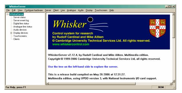
The WhiskerServer program must be running at all times when you wish to use the operant chambers. It is this program that actually communicates with the hardware.
