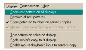
Show test pattern on all displays. Displays a test pattern on all display devices that are not in use by a client.
