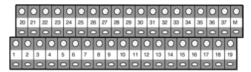
On the screw terminal assembly, terminal M is connected to the shell of the D-type connector (which, on the PCI224 itself, is connected to the computer's chassis ground). Terminal C (which may be present to the left of terminal 20 - not shown above) is not connected.
