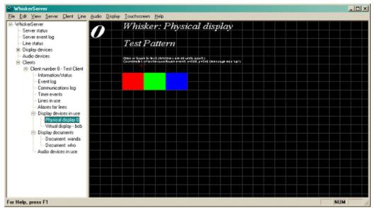
The same view, but with 'Scale server's copy...' switched on. The scroll bars have gone and the display has been shrunk to fit the server window. This allows you to see everything that is happening on a display device.
