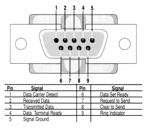
Serial ports can be configured to use the 4 **modem status lines** of a standard serial port (CTS, DSR, CD, and RI) as digital inputs.
