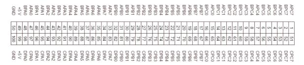
Internally, the card has four 82C55 chips, each with 24 digital I/O lines. The card is addressed in terms of 12 ports, each with 8 digital I/O lines; each port is configured as a whole for input or output.
